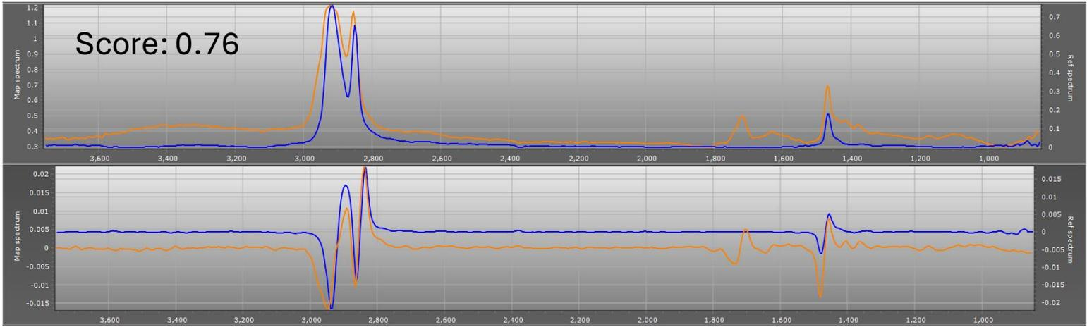
This is a PE particle with a nice fit to raw spectrum and 1<sup>st</sup> derivate
