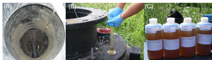
Figure 1. Example sample collection for this national landfill leachate study. (A) Manhole access to leachate stream, (B) Leachate sample collection using filter, and (C) Leachate filled bottles for sample analysis. Photographs by Dana W. Kolpin (U.S. Geological Survey).
