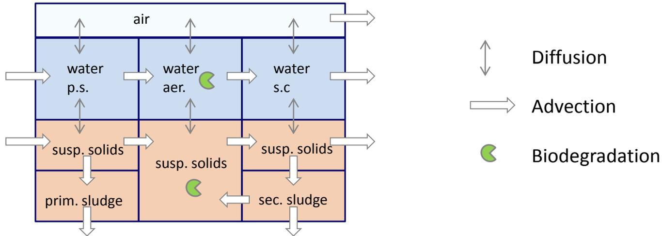
Mass balance system of 9 linear equations solved at steady-state ( $dC/dt=0$ )
