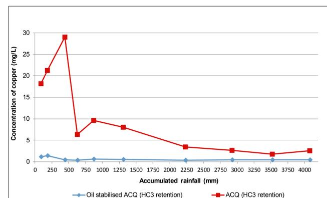
Cumulative quantity of Cu leached/m<sup>2</sup> as a function of accumulated rainfall
