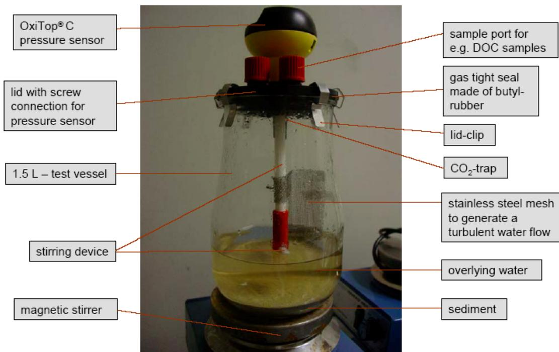
A new water-sediment test system designed to provide realistic degradation rates for polar compounds
